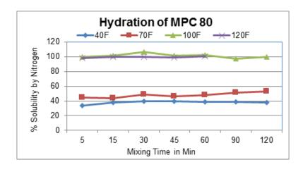
At standard HTST pasteurization temperatures, a well dispersed and well hydrated milk protein dispersion should reach maximum solubility within 5 minutes. At UHT pasteurization temperatures, the protein powder will reach maximum solubility almost instantaneously. Therefore, by the time the RTD mix has been pasteurized and sent to the filling line, the powder should be solubilized to the maximum possible.
